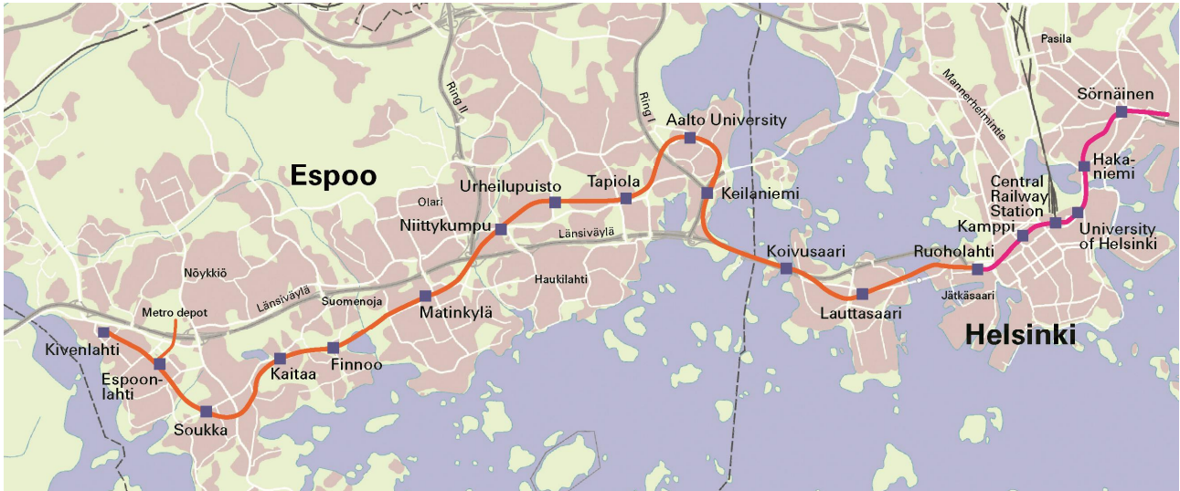
Figure 1: The West metro line, shown in orange, extends from Helsinki to Espoo. The first phase from Ruoholahti to Matinkylä is already in operation. The second phase from Matinkylä to Kivenlahti is under construction. [image source: https://www.lansimetro.fi ].
